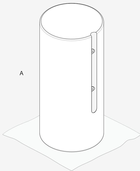
**2** Screw in rod (K) into base (A) with the provided m5 allen key screws (C). Ensure the rod remains upright (fig 2.1) when fastening the screws all the way into marble base (fig 2.2).
