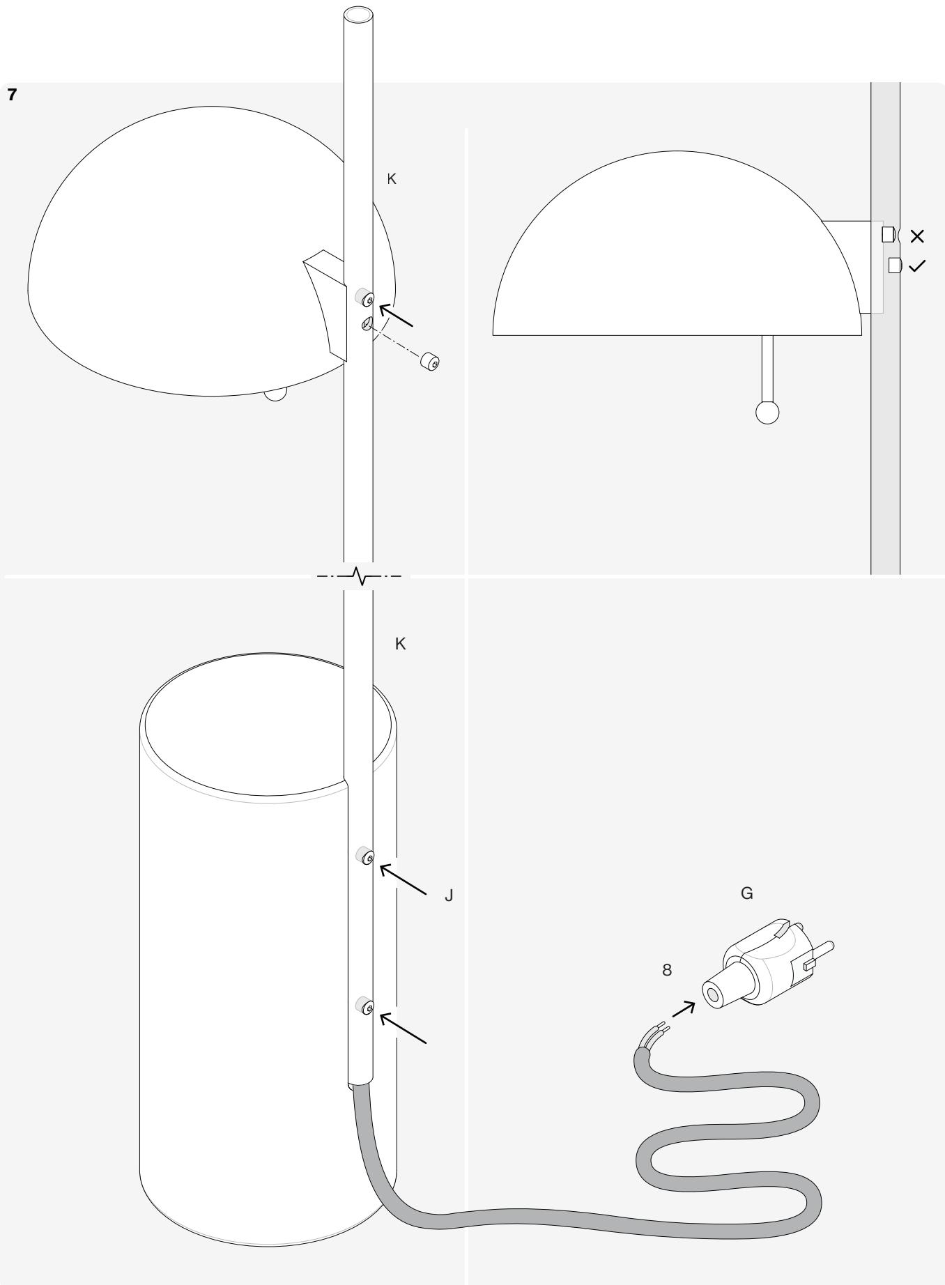
8 Open the wall plug (G) and connect the exposed cable from the bottom of the rod (K) as illustrated.
