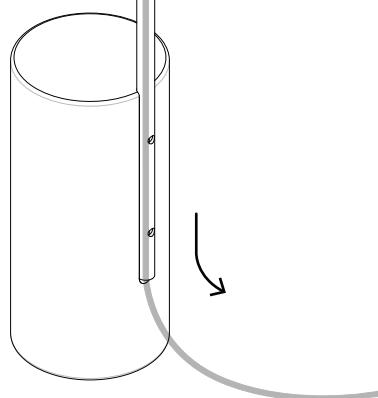
**5** Join the plug from the dimmer assembly (D) to the plug from the connection wire (H) while passing the wire through the dome (B) as illustrated (fig 5.1).
